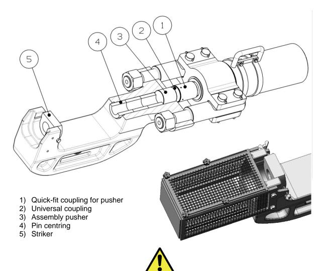
Assembly equipment parts must be requested from TRACK ONE. Do not use self-built parts. Prior to use, make sure that the parts have been set up correctly.
