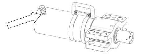
2) Fit one of the fittings into one of the two hoses on the cylinder quick-fit coupling, and its other end onto one of the two quick-fit couplings on the manual pump or electric power unit..
