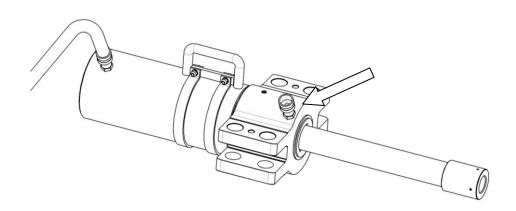
5) Detach the hose from the bottom-side and fit it onto the rod-side of the quick-fit coupling
