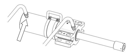
7) Make the rod retract completely, expelling all of the air contained in the hose with it
