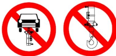
**Le piston TRACK ONE NE DOIT ABSOLUMENT PAS ÊTRE UTILISÉ COMME ORGANE DE LEVAGE**
